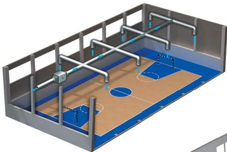
VS fan gym ventilation example.
