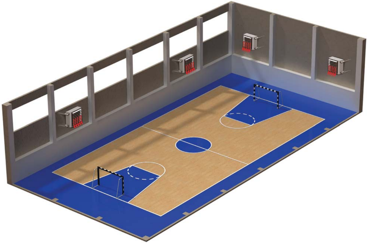
AOW heating unit gym heating example.
