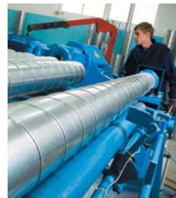
Spiro ducts workshop
