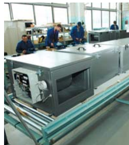
Air handling units assembling workshop
